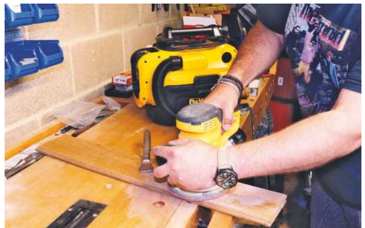
▲ Linked to power tools it does a good job of containing dust
